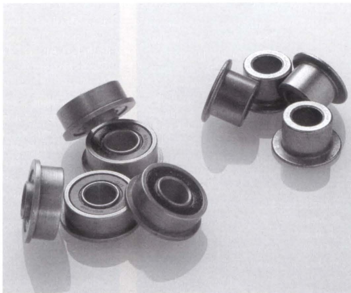
Figure 1. The heart of the enlarger improvements are provided by four flanged roller bearings and four flanged bronze bushings. These replace the original plastic bushings on the enlarger to provide much smoother head motion and more stable alignment. See parts list on page 23 for details.
