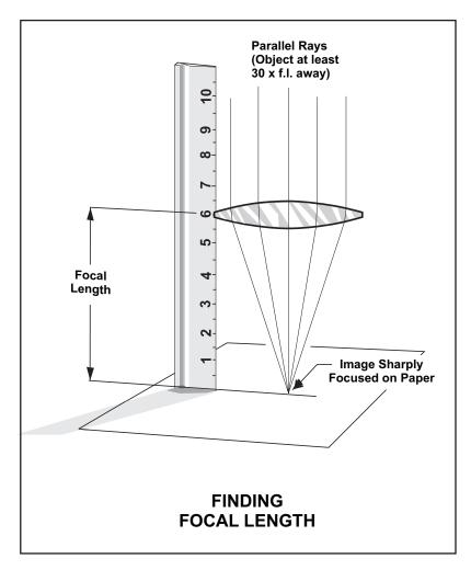
The focal length of a simple dime-store lens can be estimated easily by using a ruler and a light bulb across a room. The focal length is simply the distance from the lens to the projected image of the light bulb.
