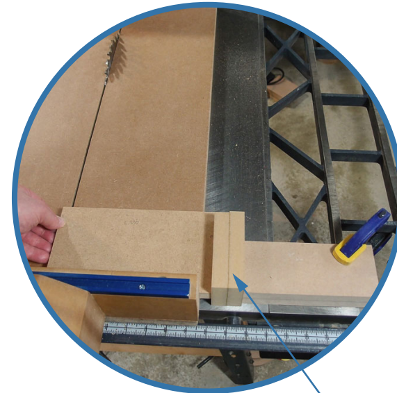
Two MDF "shims" against stop block (See step #4)
